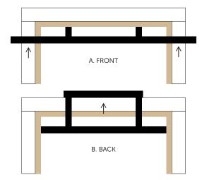
How it works? On the front side (A.) the metal pull-up bar rod rests against the door trims and on the backside (B.) the wooden pull-up bar structure rests on the upper door trim. During exercise the user's body weight presses both sides of the pull-up bar against the wall creating a solid fixation.
